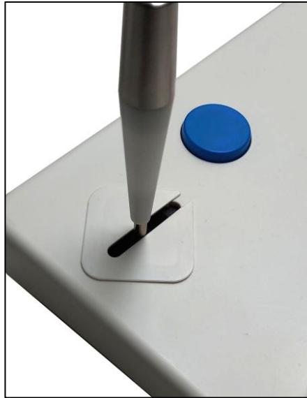
Figure 13 Joystick guide attached to the UH panel
