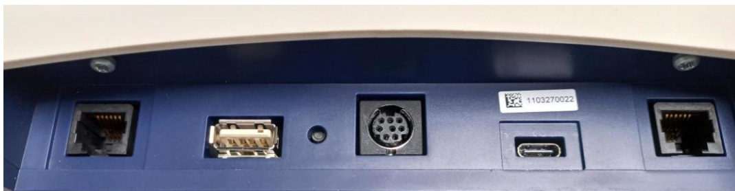
Figure 59 Connection options for the panel from left to right: RJ-45 (currently not used), USB-A port, foot-operated keys/foot pedals, USB-C port, RJ-45 (currently not used)
