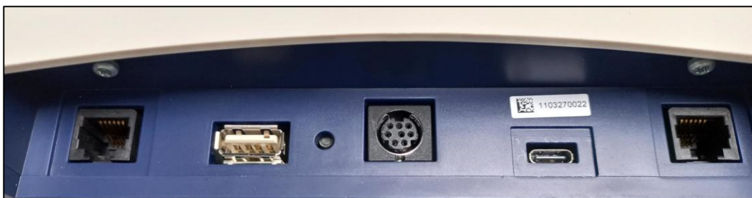
Figure 11 Connection options for the Response Panel from left to right: RJ-45 (currently not used), USB-A port, foot-operated keys/foot pedals, USB-C port, RJ-45 (currently not used)
